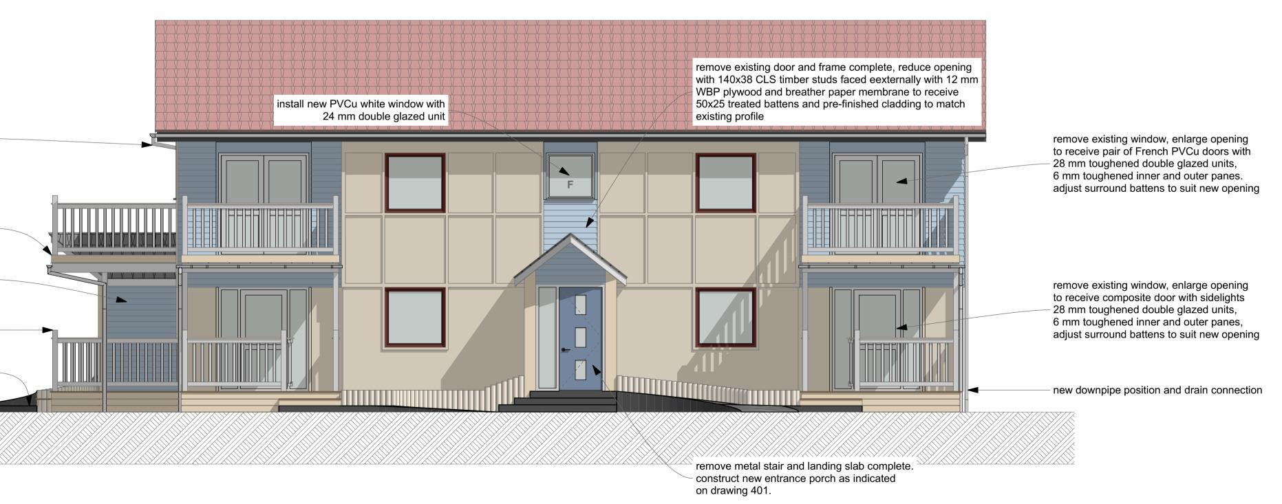
remove existing rainwater gutters and downpies complete. Replace with new rainwater goods as Marley Deepflow gutter in white with 68 dia. downpipes. Any downpipes that clash with a balcony are to be relocated to the gable or suitable new position including adaptation of the below ground drainge
