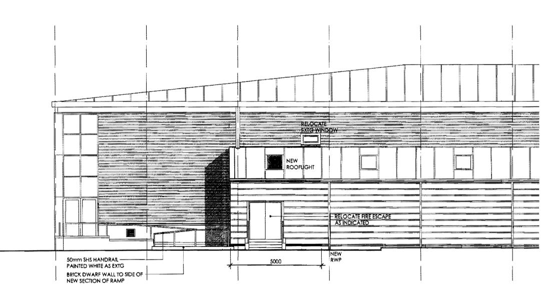
PART PROPOSED SOUTH ELEVATION 1:100
